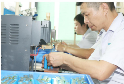
组合点焊 Combination and welding
